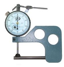
Part #FC2 Tube wall thickness
