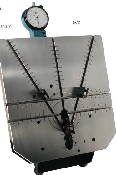
Note: Special ratio 4:5 dial indicator or electronically compensated digital indicator is recommended for 3 point non-diametric contact arrangement. See page 57 for optional indicators.
